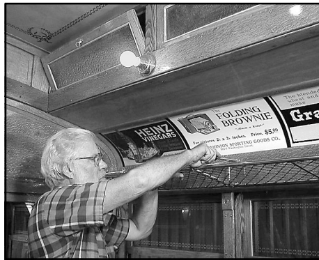
Rich Berens installs an overhead parcel rack in the No. 25. – Photo © Darrell Arndt.
